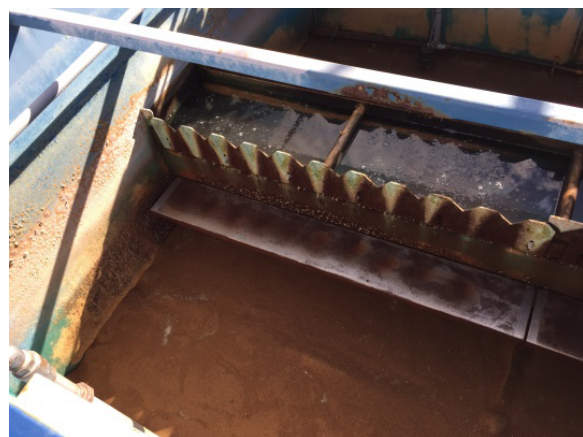
Filter bed corrosion and wear
