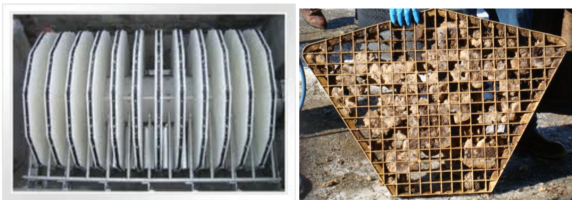
Figure 7: Cloth Disc Filters (left) and Bryozoan Sponges in a Cloth Media Filter Panel (right)
