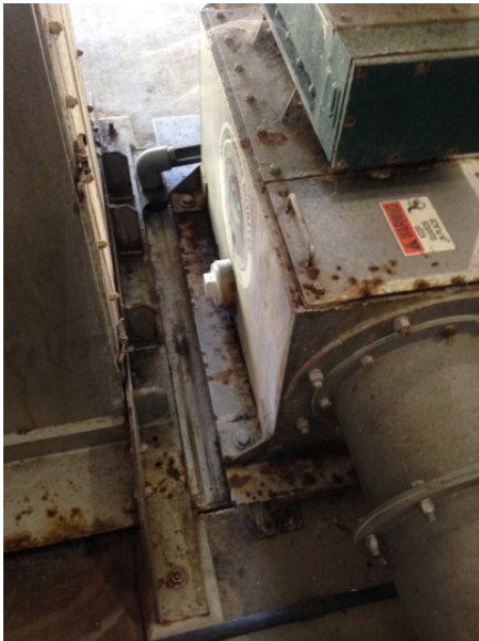
Corrosion on wash/press
