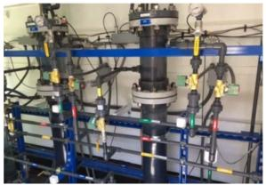
Figure 9-3. Pilot Study Filter Test Column Units setup.
