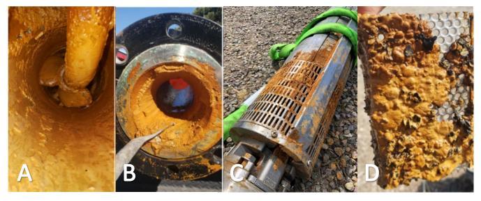
Figure 9-1. Iron and Manganese fouling of the Desalter Test Well. A) Iron fouling of propeller style flow meter. B) Iron fouling deposits in discharge piping. C) Iron fouling on test pump intake. D) Iron (orange) and Manganese (black) fouling on screen located in discharge piping.
