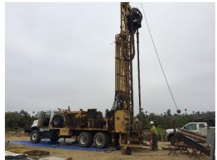
Figure 2-1. Sonic drill rig.
