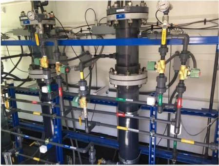
Figure 1: Filter Test Column Setup
