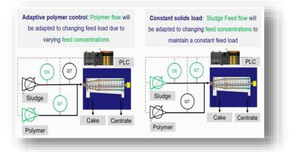
Solids Load & Adaptive Polymer Control, with the long-term objective of developing a self-optimizing decanter.
