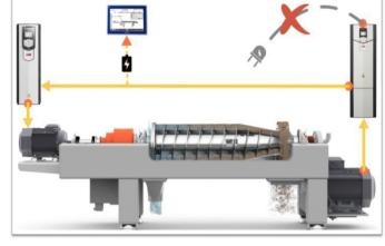
brought to a stop in a normal shutdown mode (as if it had power) maintaining the differential speed during the coast down period. This system will allow the centrifuge to scroll the solids out and be available for an immediate restart once power is restored. <u>Click on the image to see how it works</u>
