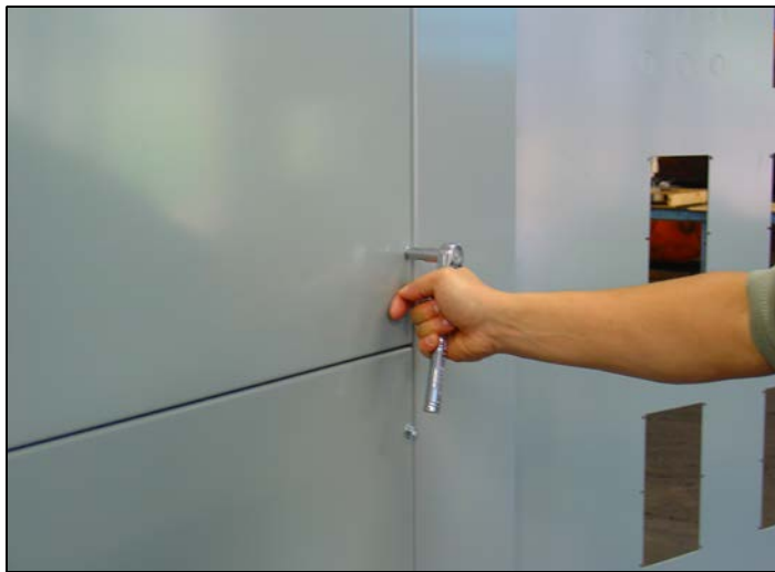
Figure 40. Removing the Bolts.
