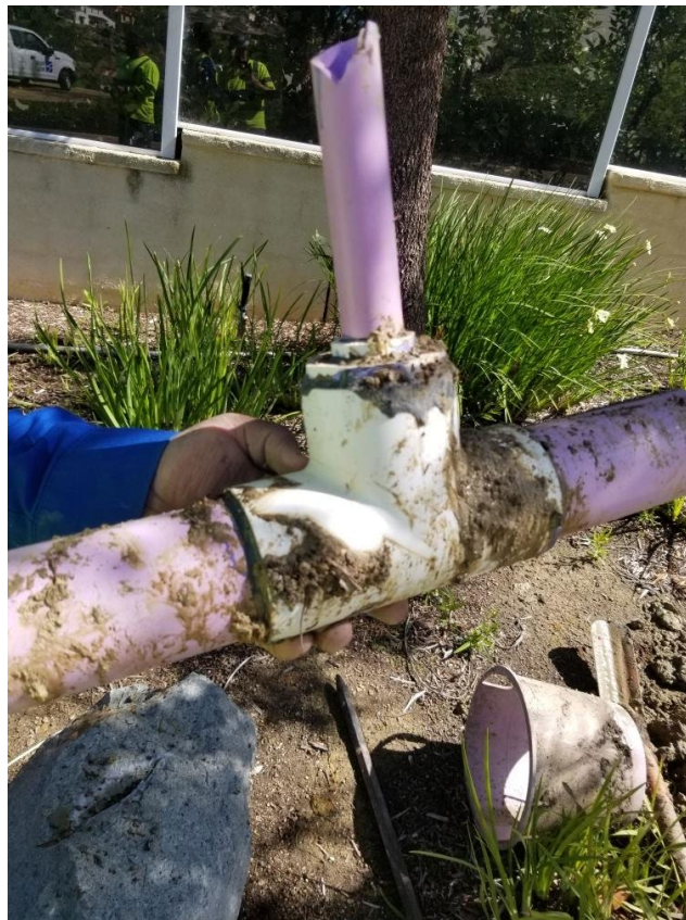
Lakes HOA Broken Irrigation Tee
